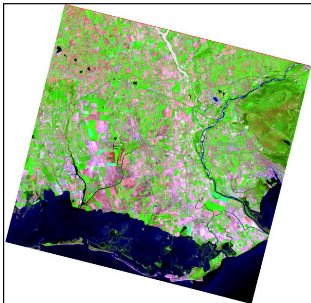
Figure 1: PRISMA SWIR-geology composite generated with i.hyper.import . Data source: PRISMA Product © Italian Space Agency (ASI), used under ASI License to Use.
