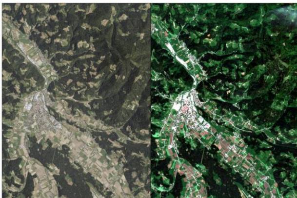
Figure 2. Orthophoto (left) and Sentinel-2 image (right) - Copernicus Sentinel data (2022) - of the same area acquired on the same day.
