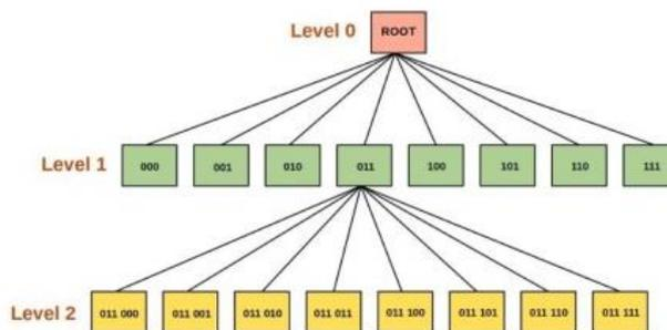
**Figure 6.** Octree organization of the voxelizing technique (Saglam et al., 2020)
