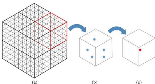
**Figure 4.** (a) 3D uniform voxel grid structure; (b) a voxel and the points located in it; and (c) one estimated point left after data downsizing (Wang et al., 2015)
