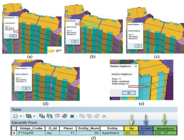
**Figure 1.** 3D unit with queried adjacent units based on close proximity analysis (Emamgholian et al., 2021).
