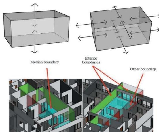
**Figure 2.** Propagated vertical and horizontal rays with resulting legal boundaries of 3D units (Barzegar et al., 2020).
