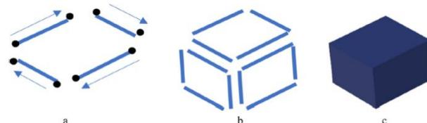
**Figure 3.** 3D volumetric parcel structure composed of (a) 3D nodes and lines, (b) 3D face and (c) 3D parcel (Jaljolie et al., 2021).
