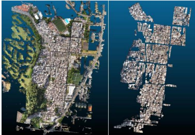
Figure 3: Left: Point cloud covering entire area, Right: Filtered point cloud only with building footprints
