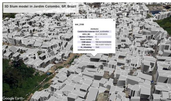
Figure 7: The final 3D model of the buildings in the slums updated with the semantic information
