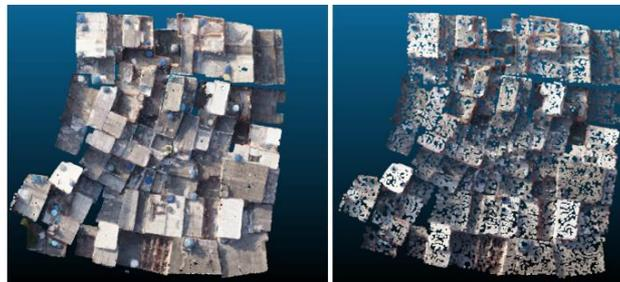
Figure 4: Left: Original point cloud with water tanks and roof furniture, Right: Filtered point cloud eliminated the waters tanks and outliers from the roof
