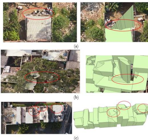
Figure 8: Errors in the 3D reconstruction of buildings in the slums : a) Erroneous spikes on the edges of the building, b) Error in the 3D building generation due to presence of vegetation c) Irregular roof structures
