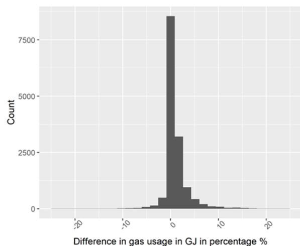
**Figure 6.** The distribution of the difference in percentage between the by Hestia calculated yearly energy demand in GJ, as a result of subtracting energy demand associated with the fully 3D approach results in from the energy demand associated with 2D & 3D hybrid approach results.
