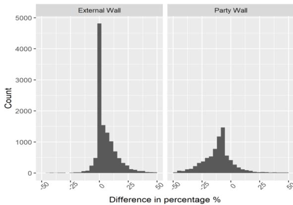
**Figure 3.** Distribution of the difference (in %) between the estimates of the external wall surface areas (left) and the party wall surface areas (right). Differences are between the hybrid and the fully 3D approach.
