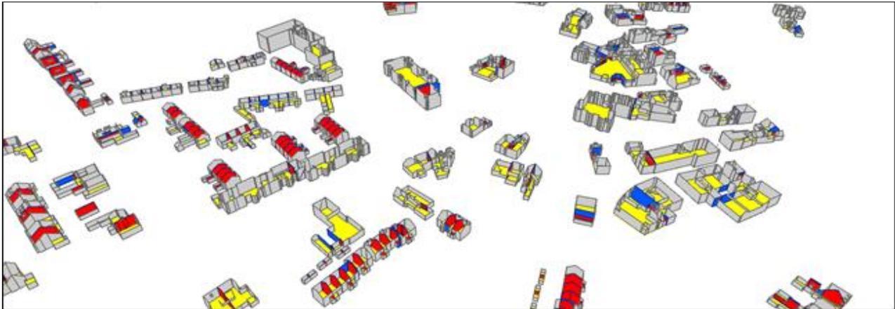
**Figure 2.** Example of 3D visualisation of the 3D city model after the computation of the party walls. GroundSurfaces are represented in yellow, WallSurfaces in grey. In case of adjacent buildings, the party walls are represented in red, while the non-shared part is represented in blue. RoofSurfaces are not shown.
