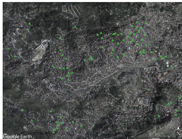
Figure 6. Sinkholes located in existing residential areas (Base map source: Google Earth, 2020)
