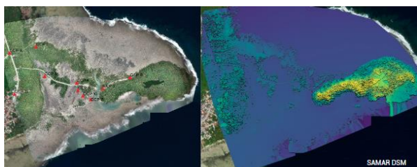
Figure 7. Orthophotos and DEM generated from drone imagery in Samar site made by Geomatics Team
