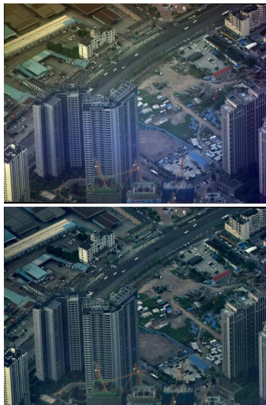
Figure 6. Comparison before and after relative radiometric correction of local radiation distortion
