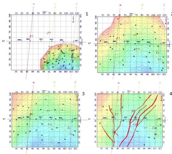
**Figure 4.** Isochron map by horizon: 1 - top of Zlatoust horizon, 2 - top of Tuskuduk horizon, 3 - top of Zhilandy horizon, 4 - top of Kopkuduk horizon.
