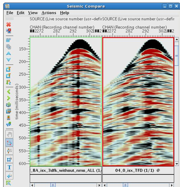
Figure 3. Seismogram before and after noise suppression.
