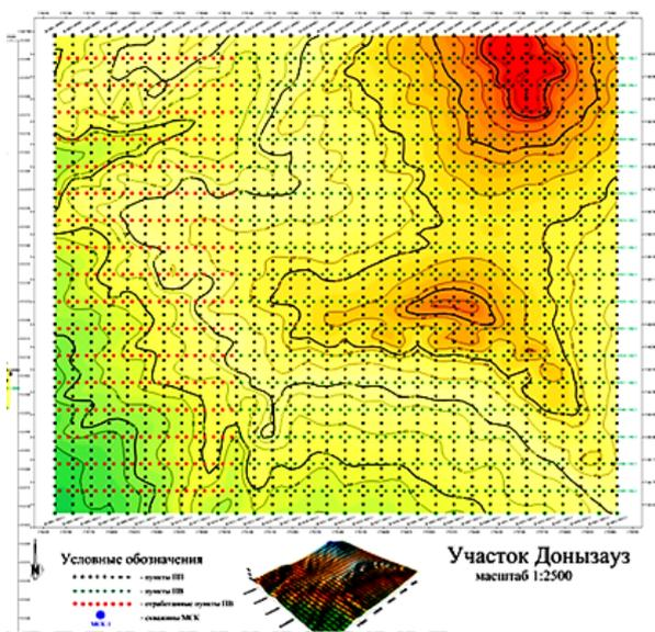
Figure 2. Point excavation diagram for experiment area of the copper sandstones group of the Zhilandy deposits.
