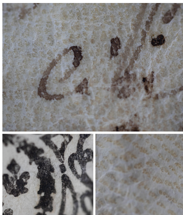
Figure 5. Composite image sequence progressively zooming into the parchment sampling area: from the calligraphic trace to the microscopic identification of the parchment substrate (optical magnification 5:1). Images were acquired by the author at Labo.R.A. – Laboratory of Architectural Restoration, Department of Architecture, University of Ferrara, using an optical bench with a Canon R5 mirrorless camera equipped with a Canon MP-E 65mm f/2.8 macro lens.
