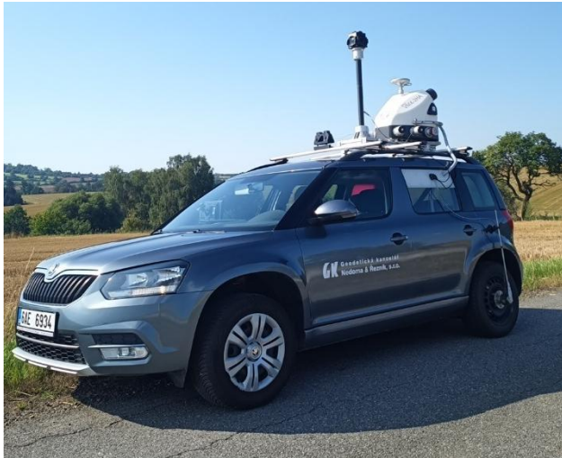
Figure 2. Riegl VMX-2HA mounted on Škoda Yeti 2.0 TDi 81kW 4x4
