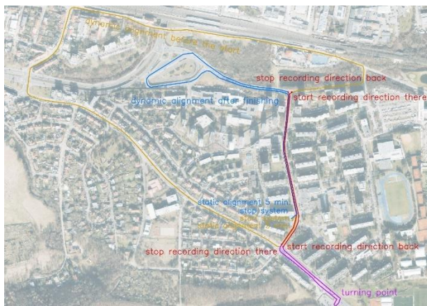
Figure 5. Data collection pass scheme
