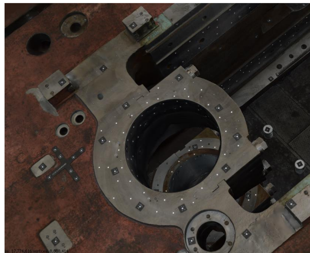
Figure 4. Photogrammetrical processing, Linearis system
