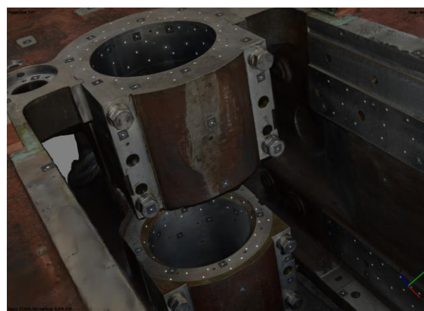
Figure 10. Detail of the 3D model created in Agisoft Metashape (pointcloud)
