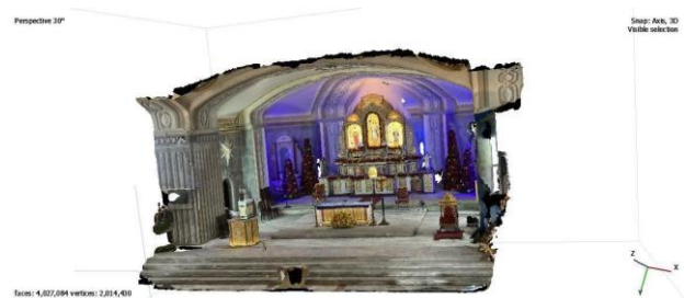
Figure 9. Textured Unrefined Model or Mesh.
