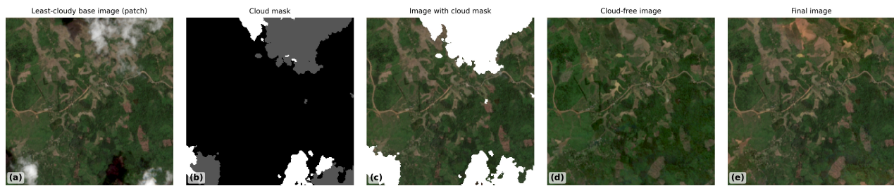
Figure 5. VPint2 cloud-minimization workflow. (a) Least-cloudy base image (patch) from March 12, 2017 ; (b) Cloud mask from OmniCloudMask: black = clear, gray/white = cloud and shadow.; (c) base image with mask applied, showing residual cloud/opaque areas; (d) cloud-free reference from July 9, 2017 (nearest low-cloud acquisition for this patch); (e) final result after applying VPint2 . Image selection was restricted to the dry season (Feb–April), and the March scene was chosen as the baseline to keep phenology and illumination consistent. For each patch, a nearby cloud-free observation (here July 9) was used only as a donor. Rather than stitching, VPint2 transfers brightness, hue, and local texture from the donor to the base so infilled areas match the base image.
