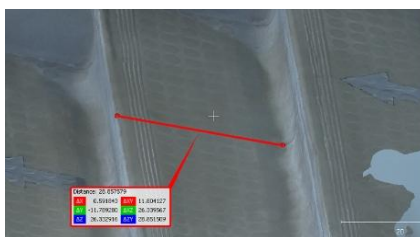
Figure 5. Sample image of the measurement of the tread using CloudCompare.
