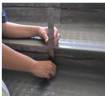
Figure 6. Sample image of the actual rise measurements using a metal ruler.
