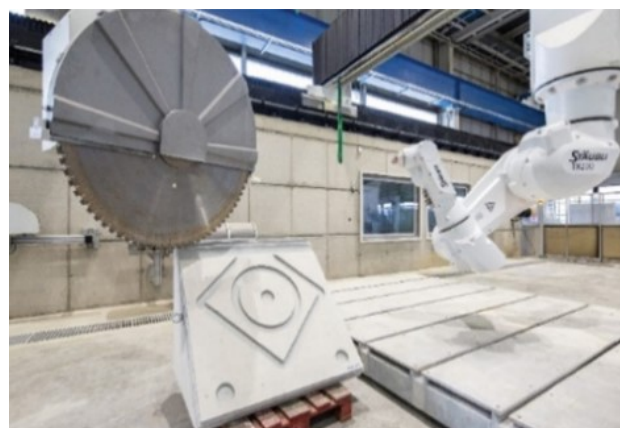
Figure 1. Digital fabrication of a concrete component (Hack et al., 2022)
