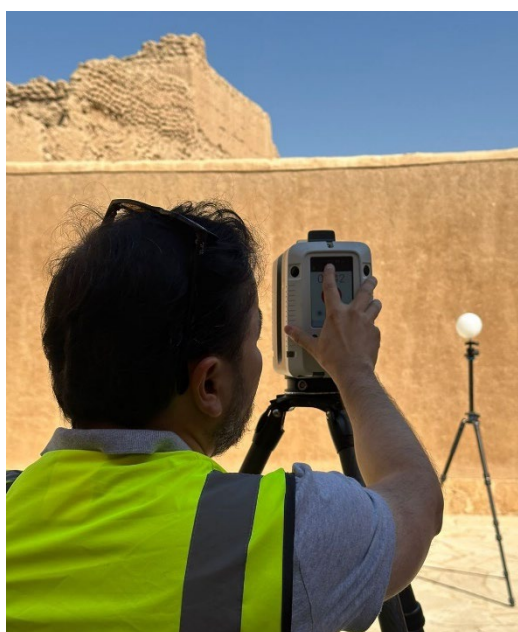
Figure 5. using 3D laser scanning (Leica RTC360) on site(Ref. A.Baik).
