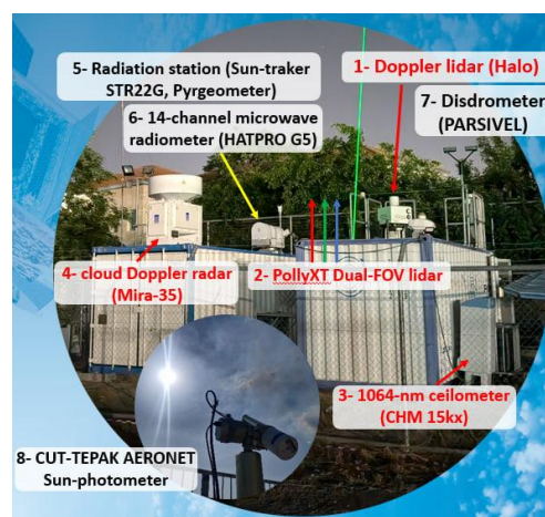
Figure 2- The main ground-based multi-instrument facility of the Cyprus Atmospheric Remote Sensing Observatory (CARO), hosting both active and passive remote sensing instruments, is located at 34.677° N, 33.0375° E, at an elevation of 2.8 m above sea level.
