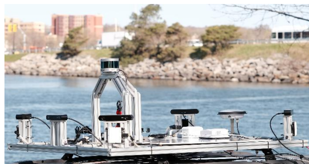
Figure 2. Multi-sensor platform – 4 corner stereo cameras, one forward-looking stereo camera, one mechanical LiDAR, and a GNSS receiver integrated with high-end (reference).
