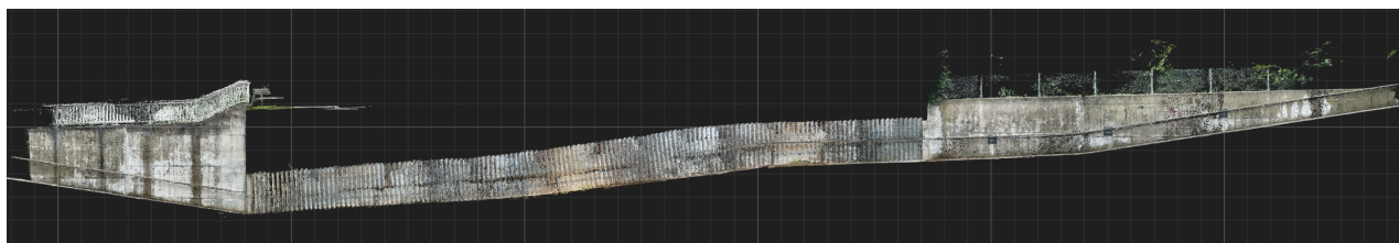
Figure 4. Screen capture of PIX4Dmatic showing the side profile view of the tunnel. Major grid cell: 10 \times 10 m, minor grid cell: 1 \times 1 m.
