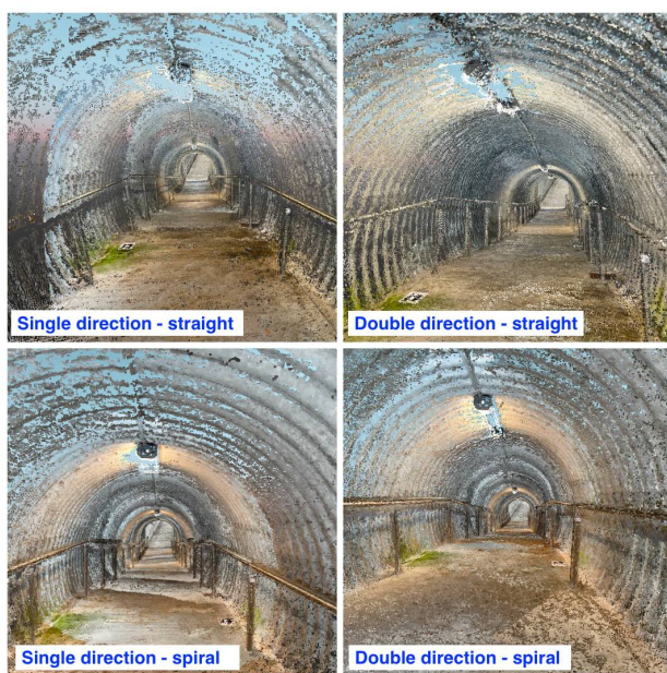
Figure 6. Visual comparison of the fused point clouds (dense point cloud + LiDAR) for the four scanning patterns detailed in Sec. 2.3.1.
