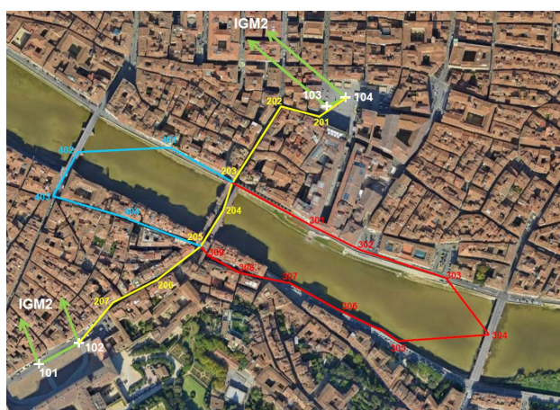
Figure 1. Diagram of the geodetic control network. The main network points (in white) are defined in relation to the GNSS permanent station IGM2 (in green). The densification networks are shown in yellow, red and blue.
