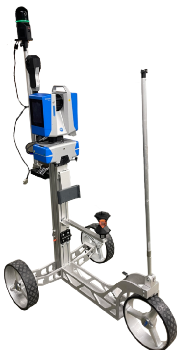
Figure 6. Designed scanning platform.
