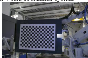
Figure 2. One example of the checkerboard image acquisition by this trinocular camera system
