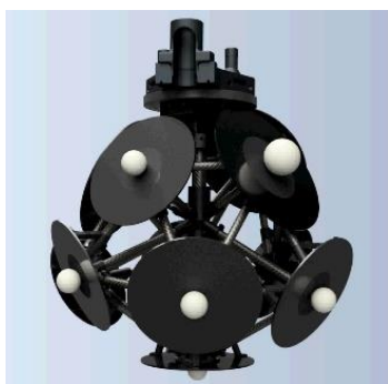
Figure 5. CAD model of the spatial encoded target artefact prototype
