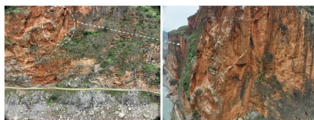
Figure 1. Typical examples of hazardous rock masses and rockfalls triggered by joint formations surrounding the studied rock slope.
