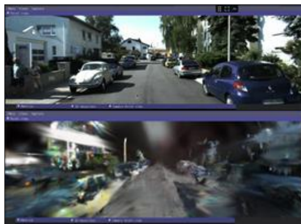
Figure 1: Forward (top) and backward (bottom) Gaussian Splatting render of a KITTI image set, showing poor photorealism in the backwards render.
