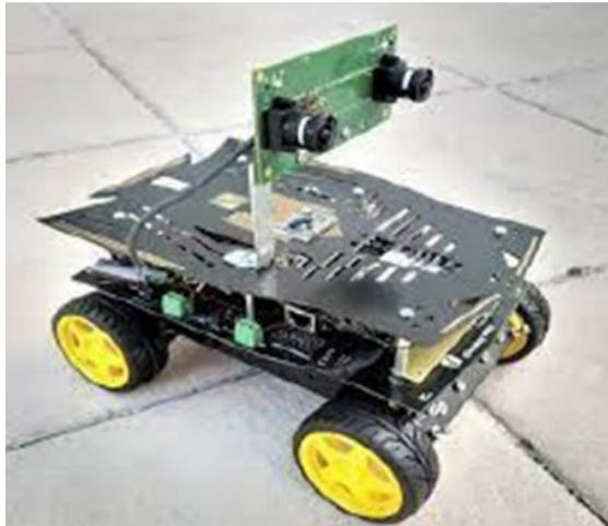
Figure 2. A pair of stereo cameras mounted on mobile robot (Yaqoob and Bajwa 2024).
