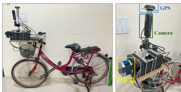
Figure 1. A specialised data collection setup mounted on a bicycle.
