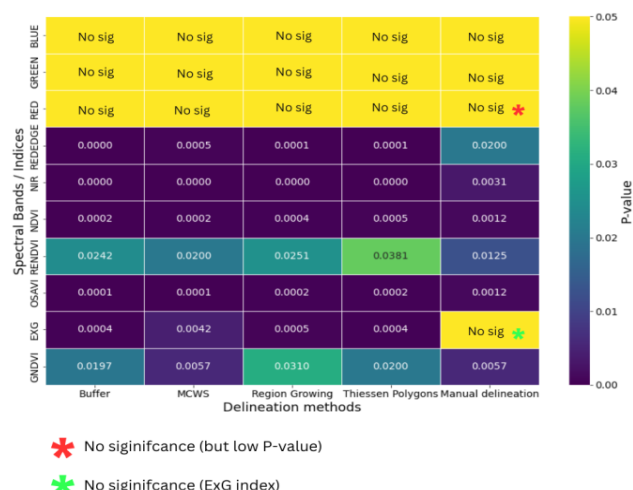
Figure 6. Heatmap of the spectral separability (between healthy and infested trees) for each delineation method (Automatic and manual) across different spectral features. (No sig: No statistical significance)
