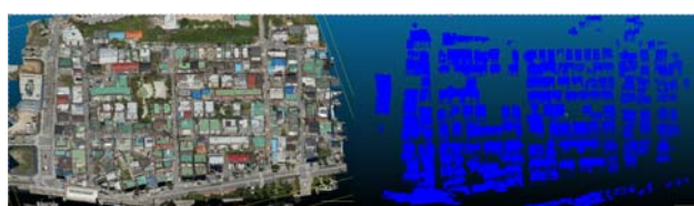
Figure 14. Before and after applying tree removal and height-filter
