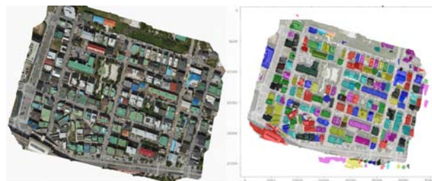
Figure 15. Building candidate extraction using DBSCAN clustering algorithm
