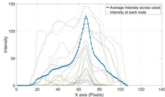
(b) Intensity value across the crack and Average intensity value across the crack of an estimated crack width of 8.4 mm
