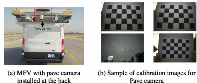
Figure 1. System configuration and calibration data
