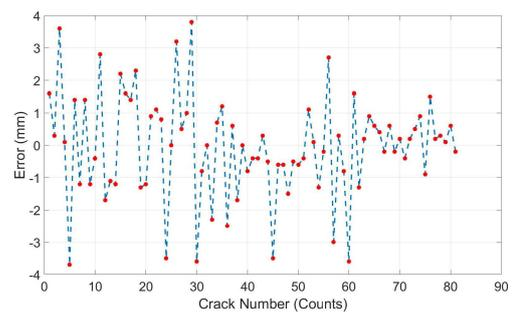
(e) Error of estimated crack width for total 82 cracks
