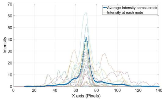
(a) Intensity value across the crack and Average intensity value across the crack of an estimated crack width of 5.8 mm
