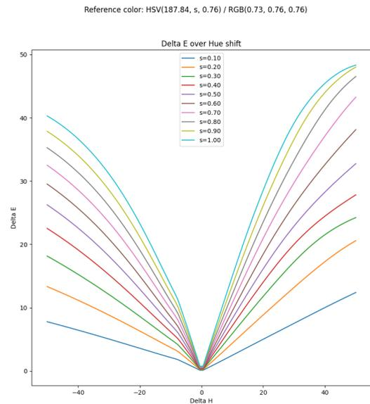
Figure 8. Plot of  $\Delta E$  vs.  $\Delta H$  for a reference concrete color (HSV: 187.84°, s, 0.76) over multiple values of  $S$  from 0 to 1. This shows the strong dependence on the saturation.
