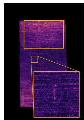
(b)  $\Delta E$  of the image shown in Figure 6 with the two anomalies highlighted.
