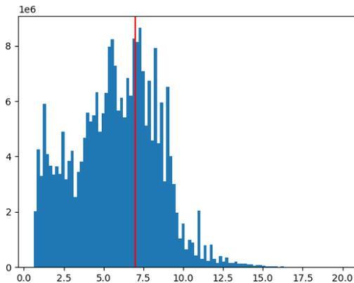
Figure 7.  $\Delta E$  distribution of the red panel reference image. The vertical line marks the threshold of 7.
