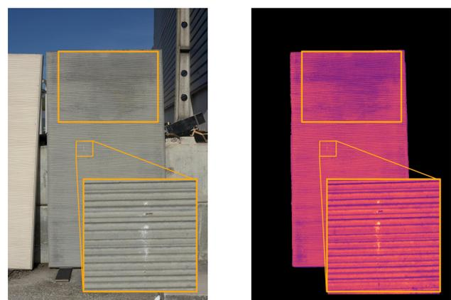
(a) Two identified regions of significant  $\Delta E$  derivation, marked in orange.
