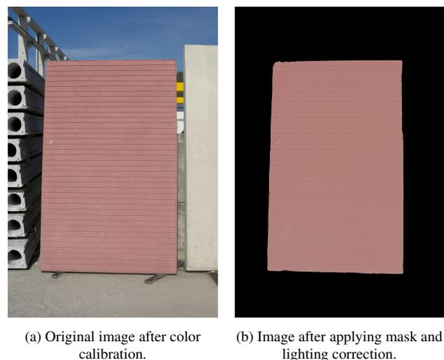
Figure 4. The effect of applying the lighting correction. The shadows of the structured parts are removed and the plain surface remains.
