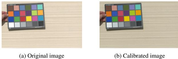
Figure 2. Calibration of the images using the color checker.
