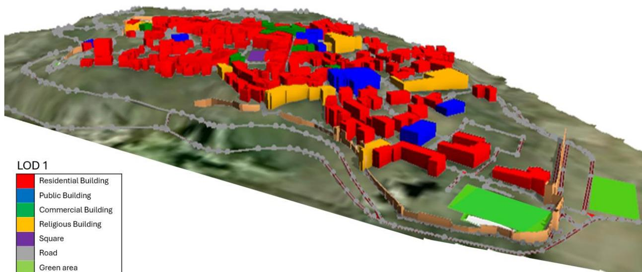
Figure 4. Functional classification of the 3D CityModel (© the authors, 2025)
