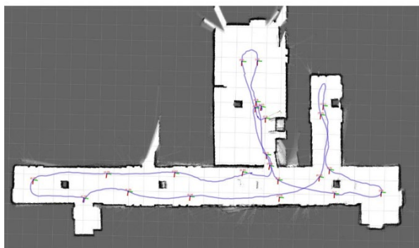
Figure 7. Real-time Generated 2D SLAM Map
