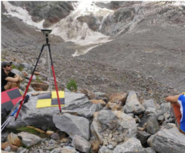
Figure 1. Image of a GCP located on the Belvedere Glacier measured with a GNSS antenna.
