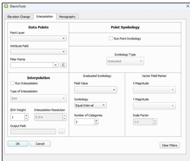
Figure 2. Example of the GlacioTools plugin GUI in the QGIS environment. The screenshot shows the Interpolation tab with the requested parameters to be defined through user input.
