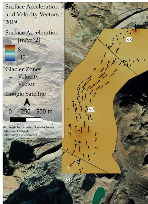
Figure 7. Example of a surface acceleration map interpolated from homologous points and GCPs in the Belvedere Glacier, 2019.
