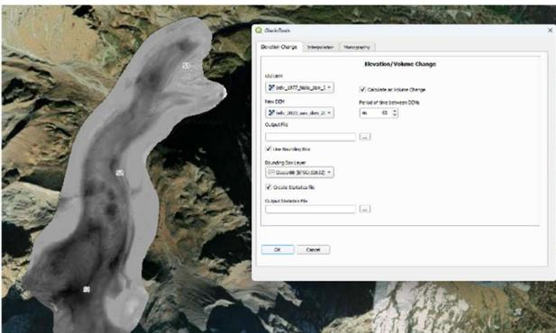
Figure 5. Example of the QGIS interface for the Elevation and Volume Change analysis within the GlacioTools plugin.
