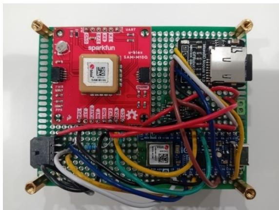
Figure 1. Basic camera interface board using a u-blox SAM-M10Q (on the red board) to get the GNSS time frame.
