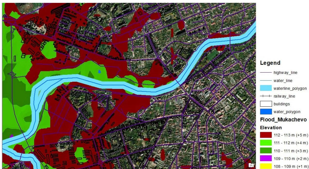
Figure 3. Digital map of predicted flooding for the city of Mukachevo based on the winter image (Fig. 2a) as a result of our study.
