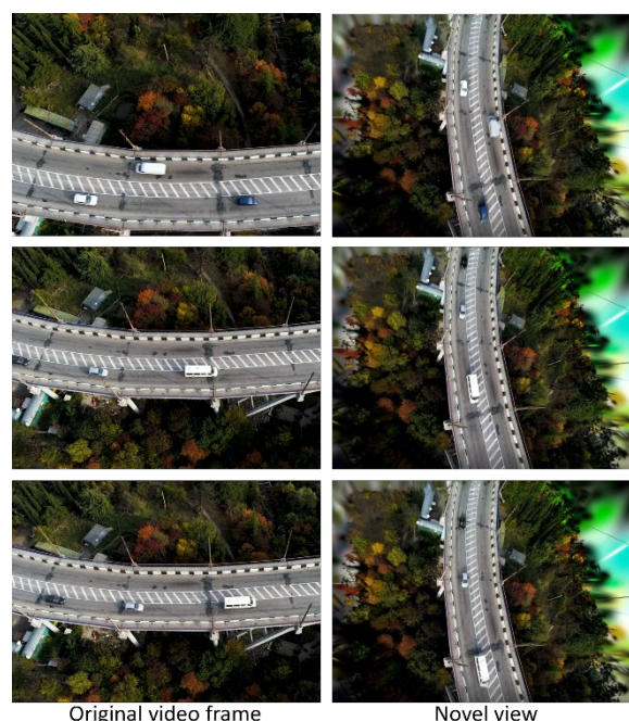
Figure 5. A stationary and global viewpoint synthesized from the viaduct footage, revealing moving vehicles more clearly and showcasing the effectiveness of the proposed pipeline.
