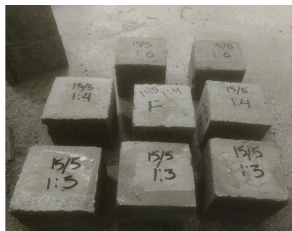
Figure 3. Mortar Samples prepared in the laboratory. Moulding date and mix ratio are indicated over the samples.
