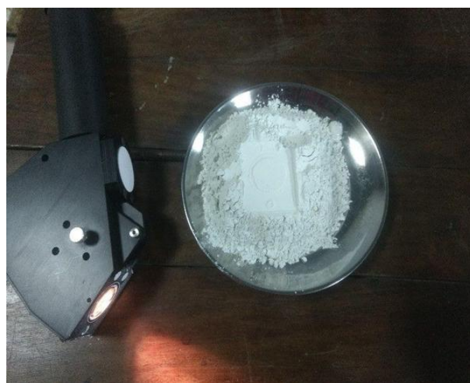
Figure 1. A spectroradiometer and a sample of WPC were used for testing.
