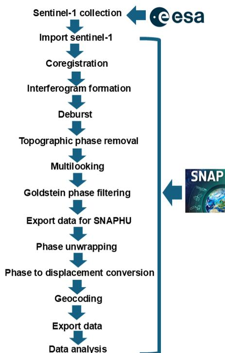
Figure 3. Flowchart of vertical land displacement analysis on Sentinel-1 images using SNAP software developed by ESA.
