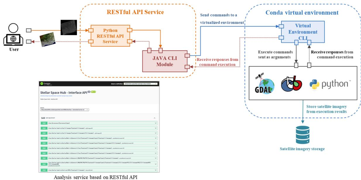
Figure 2. Architecture of the web-based analytical system for satellite data processing and visualization
