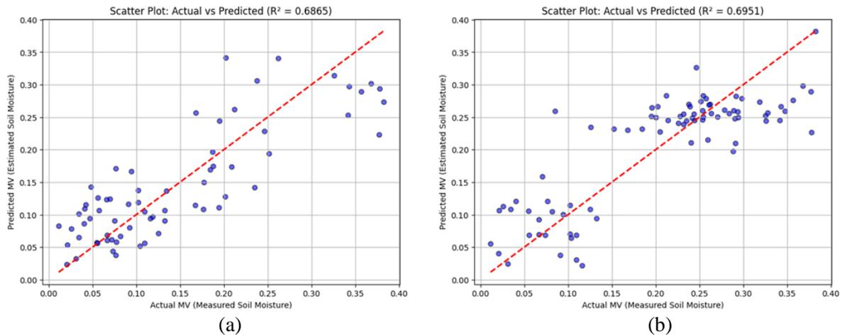
Figure 3. Scatter plots of soil moisture estimation using WCM: (a) RVI-based WCM, (b) NDWI-based WCM.
