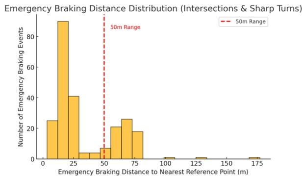
Figure 11. The emergency braking distance distribution
