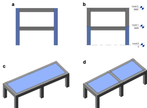
Figure 3. How columns and slabs should be included in the model. Incorrect way of representation of columns (a) and slabs (c), Correct way of representation of columns (b) and slabs (d)
