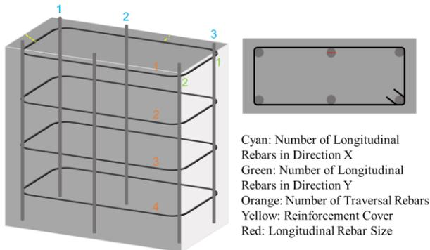
Figure 2. Information provided in the cross-section of a structural column, 3D View (Left), 2D View (Right)
