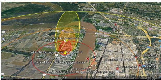
Figure 5. Georeferenced ALOHA dispersion output showing AEGL-based ethylene oxide threat zones overlaid on Google Earth imagery for the Port Allen Lube Plant. The red (AEGL-3), orange (AEGL-2), and yellow (AEGL-1) zones illustrate decreasing exposure severity with increasing distance from the emission source. The spatial overlay highlights the proximity of residential neighbourhoods, transportation corridors, and industrial facilities located within predicted impact zones.
