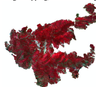
Figure 3. The cropped pseudo-color image using the near-infrared, red and green bands.
