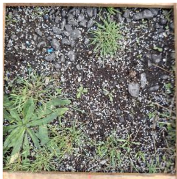
Figure 2-2-1 original smartphone RGB image, showing pellets within a wooden quadrant of 50cm by 50cm at a natural site in the port of Antwerp.
