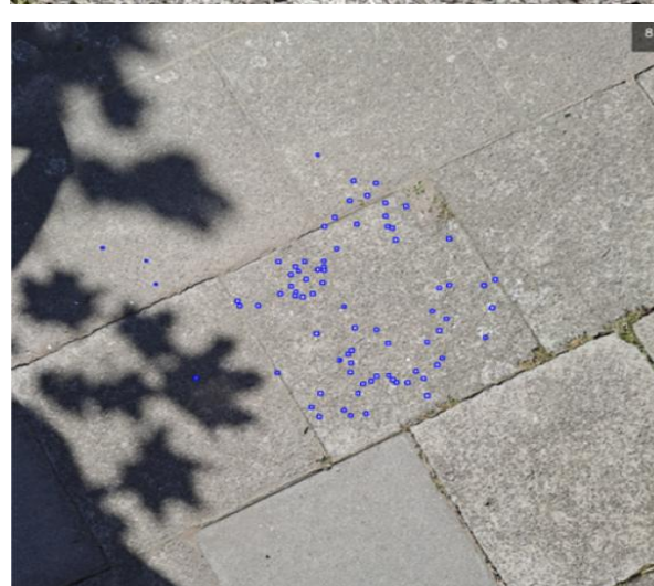
Figure 3-3 Pellets on pavement. Top: zoomed in on small area. Bottom: complete smartphone image, with detected pellets indicated with blue boxes.
