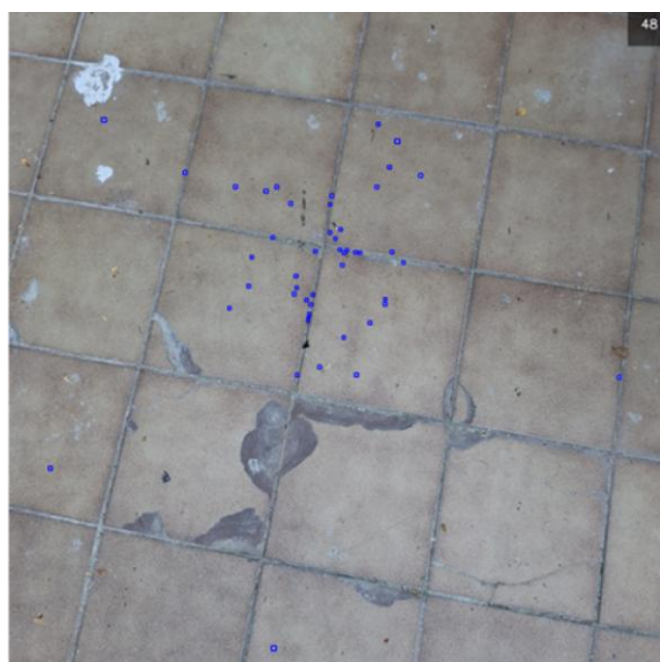
Figure 3-4 Terrace tiles Top: zoomed in on small area. Bottom: complete smartphone image, with detected pellets indicated with blue boxes.
