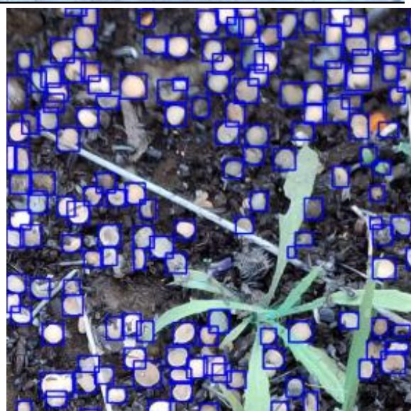
Figure 3-2 Top: object detections via a YOLO Computer Vision model over the whole quadrant; Bottom: one part of the RGB image with pellet detections denoted as blue boxes around individual items.
