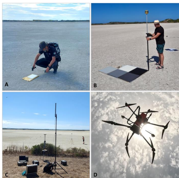
Figure 2. Field measurements and UAV hyperspectral data acquisition at Sal 'e Porcus: (A) measurement of a calibrated Spectralon white-reference panel used for the ASD field spectroscopy of the saline surface; (B) RTK GNSS survey of the five radiometric targets used for empirical-line calibration of the UAV imagery; (C) field instrumentation and GNSS base-station setup supporting the UAV survey; and (D) the customised DJI Agras T30 carrying the Specim AISA Kestrel 10 sensor during the VNIR hyperspectral flight.
