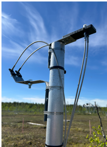
Figure 3. The FloX measurement setup at the Halssiaapa study site. Two upward-facing optical fibers measure downwelling irradiance, while two downward-facing fibers measure upwelling radiance from the vegetation canopy. The spectrometers are located in the weatherproof enclosure near the base of the measurement pole.
