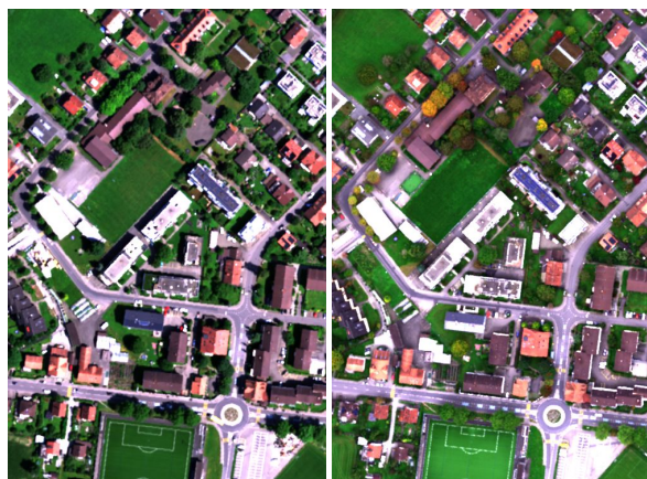
Figure 6. AVIRIS-4 data of the same area taken once under sunny conditions (left) and below fully overcast situation (right), scaled to the same brightness range; data courtesy of RSL Univ. Zurich.
